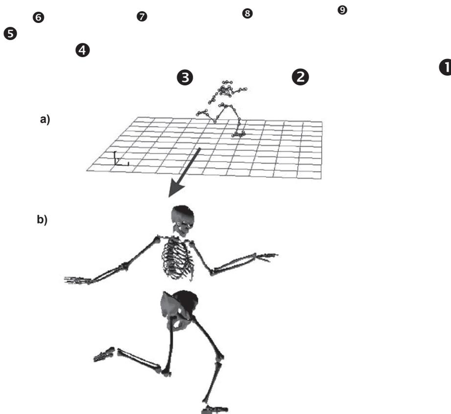
Figure 3. Maximal instep soccer kick – the set-up of 3D data collection, a sample of 3D motion capture and the 15-segment full-body model derived from 3D raw data. Each tiny circle in Figure 3a represents a marker captured. The 3D raw data contains only coordinate information. Through biomechanical modeling, the anatomical positions and markers were linked together to reconstruct a skeleton.
