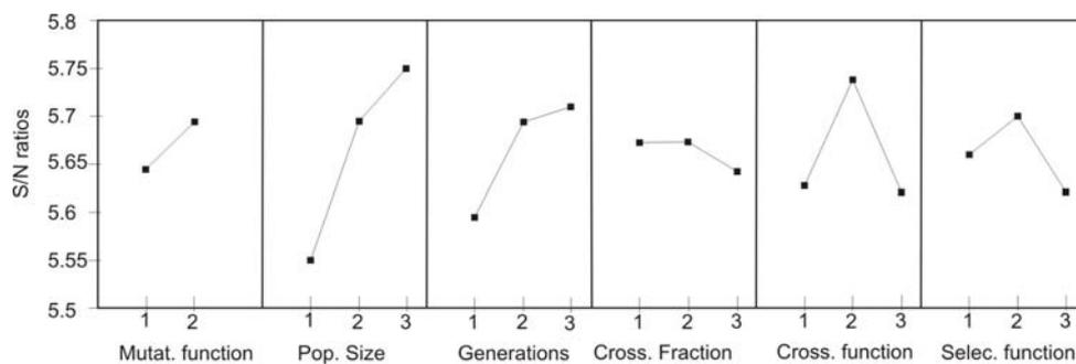
Fig. 2 The average S/N ratio plot at each level for objective values in RCGA
