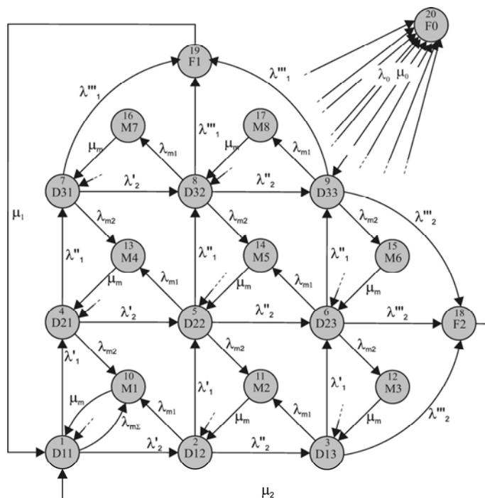
**Fig. 1** Maintenance model of a system composed of two components (subsystems)
