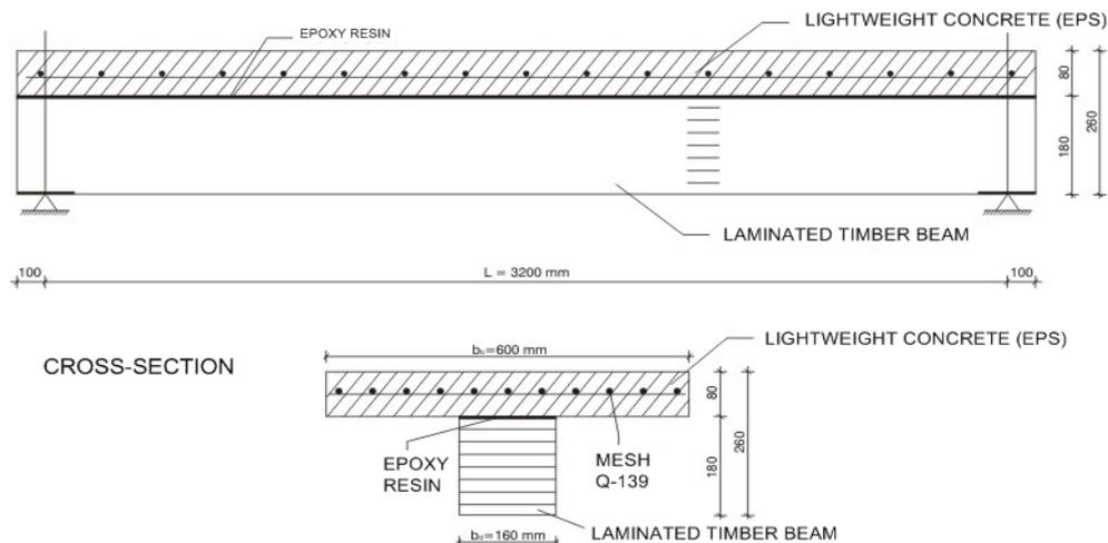
Figure 1. Tested composite timber-concrete beam specimen [2].
