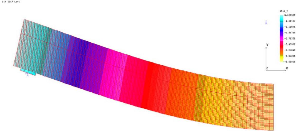
Figure 6. A finite element model for the composite timber-EPS specimen.
