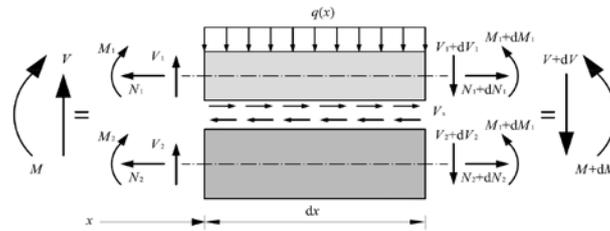
Figure 7. Equilibrium of a two-layer beam section.
