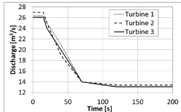
Figure 4. Turbine discharge reduction for the Scenario 1.
