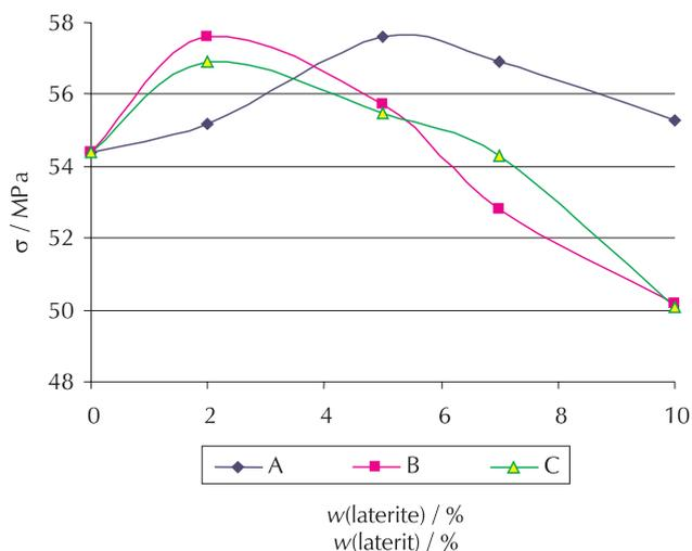
Fig. 8 – Comparison of 28 days compressive strength of OPC and laterite blends
