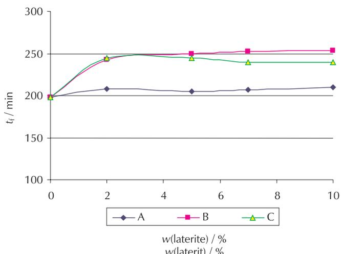
Fig. 4 – Comparison of final setting times of OPC and laterite blends
