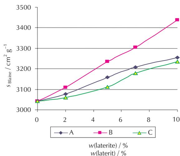
Fig. 1 – Comparison of specific surface area of OPC and laterite blends
