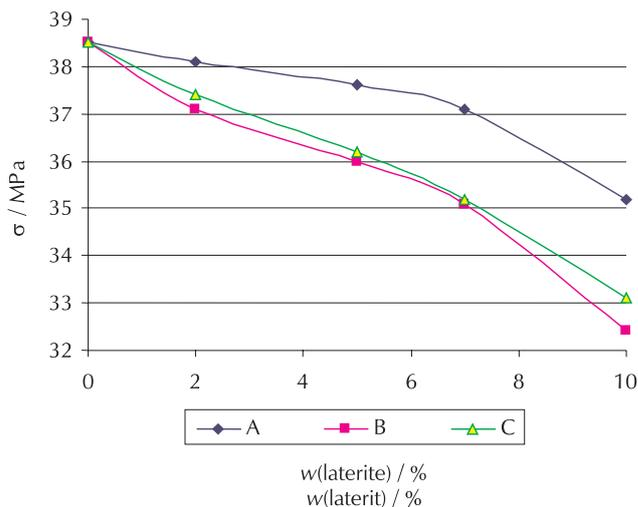
Fig. 6 – Comparison of 3 days compressive strength of OPC and laterite blends
