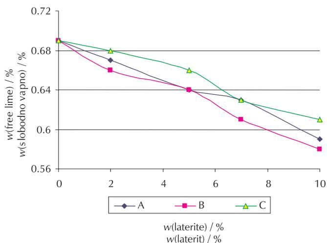
Fig. 9 – Comparison of free lime of OPC and laterite blends
