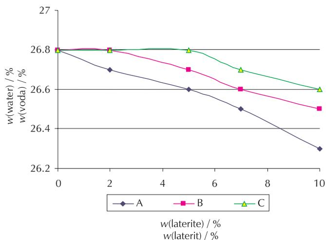
Fig. 2 – Comparison of water consistency of OPC and laterite blends
