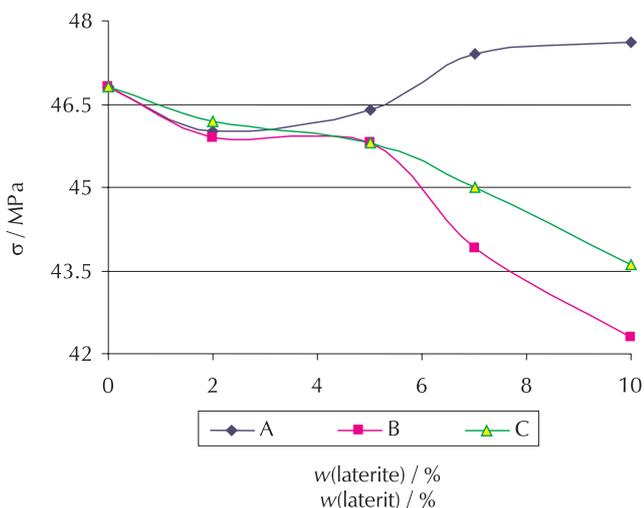
Fig. 7 – Comparison of 7 days compressive strength of OPC and laterite blend
