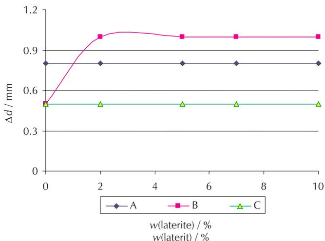
Fig. 5 – Comparison of Le-Chatelier expansion of OPC and laterite blends
