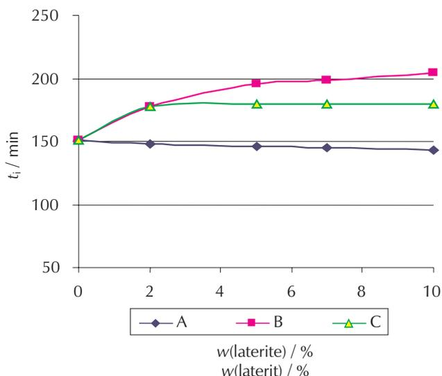
Fig. 3 – Comparison of initial setting times of OPC and laterite blends
