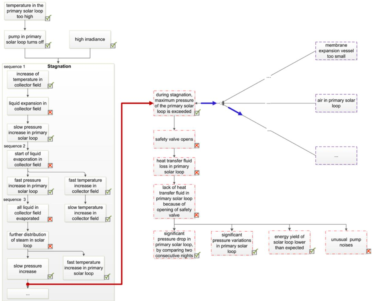
**Figure 5.** Fault situation as causal link between different events that are categorised into features, symptoms and faults according to the four step concept. Features are framed by a continuous line, symptoms by a dashed line and faults by a dash-dotted line. Events that can automatically be detected with established sensors are indicated by a check mark, others by a cross.
