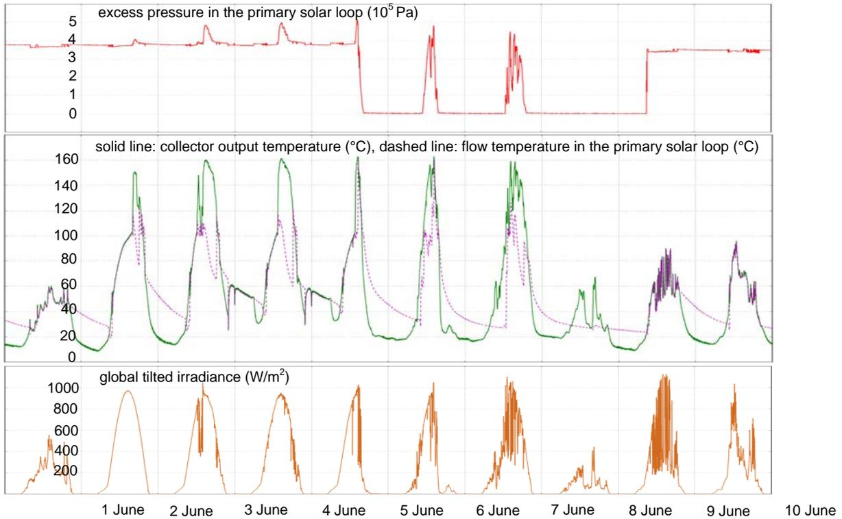
**Figure 3.** Excess pressure in the primary solar loop, the collector output temperature and the flow temperature in the primary solar loop and the global tilted irradiance between the 1<sup>st</sup> and the 10<sup>th</sup> of June 2011. The time resolution of the measured data is one minute. In this time interval the solar storage is not completely loaded.
