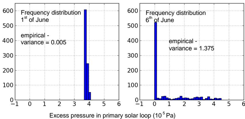
**Figure 6.** Frequency distribution and the empirical variance of the excess pressure in primary solar loop. Left: (1<sup>st</sup> of June) represents the expected typical frequency distribution of the fault free process. Right: (6<sup>th</sup> of June) represents a day with a high pressure variation in the solar loop.
