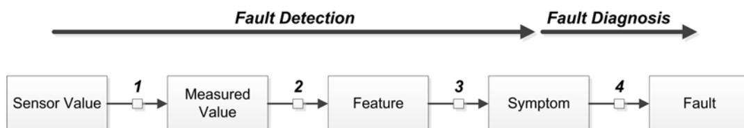
Figure 2. Four-step concept of the algorithm-based FDD.
