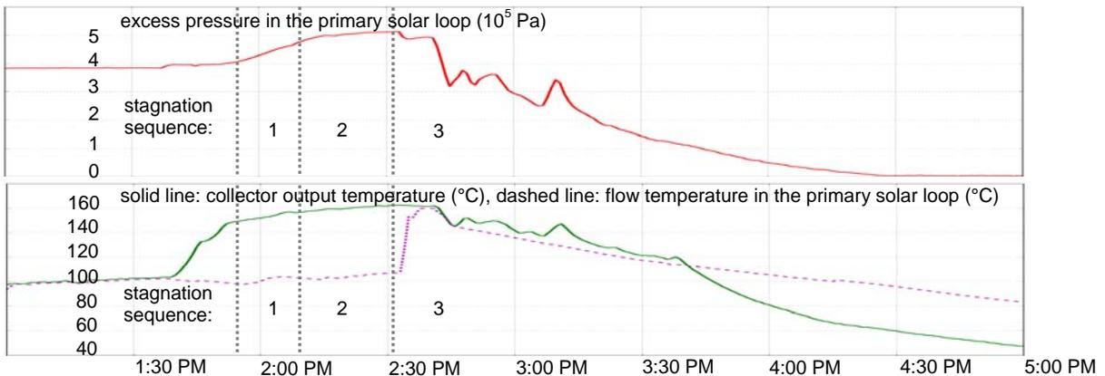
**Figure 4.** Excess pressure in the solar primary circuit, the collector output temperature and the flow temperature in the primary solar loop, 5<sup>th</sup> of June 2011 1:00 PM to 5:00 PM.
