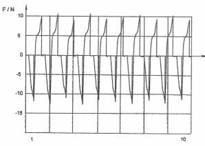
Figure 6 Retention force with added saliva - loading cycles from 1 to 10.
