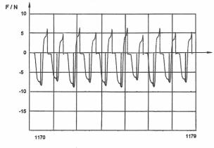
Figure 7 Change of the retention force with added saliva - loading cycles 1170 - 1179.
