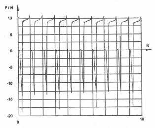
Figure 3 Results of measuring the retention surfaces force with dry touching - first ten cycles
