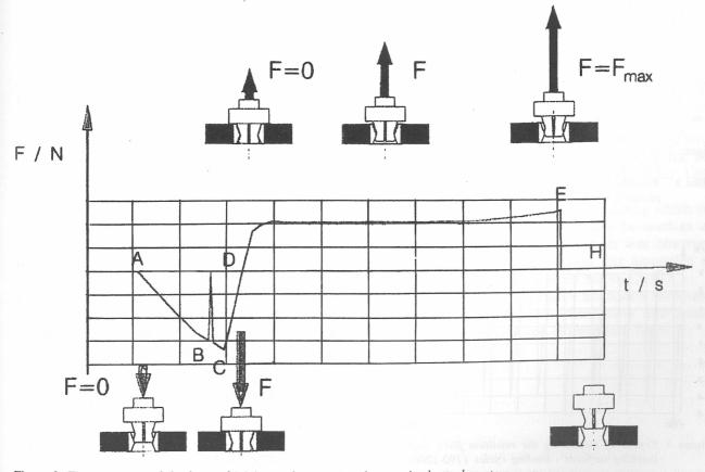
Figure 2 Time sequence of the force of joining and separating the examined attachment Slika 2. Vremenski slijed sila spajanja i rastavljanja ispitivanog ankera
