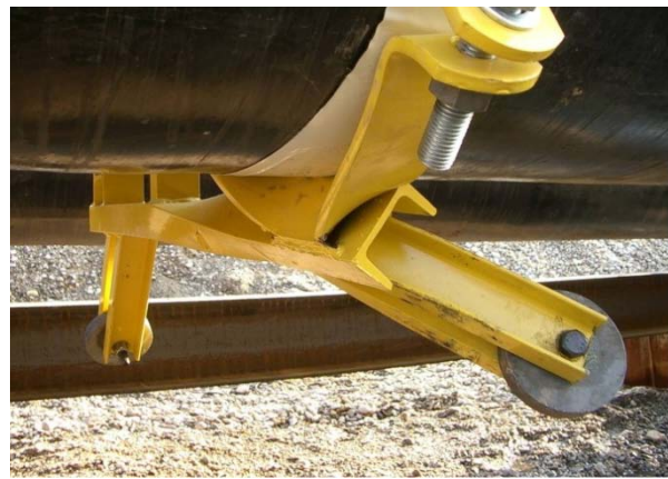
Fig. 3 Bent structure of the support
