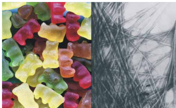
Figure 19. TEM image of ( S,S )-oxalyl-dileucinol toluene gel negatively stained by dipotassium phosphotungstate (right), and an application of gel – Haribo bonbons (left).
