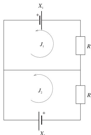
Figure 7. The electrical network with two loops and zero mutual resistance.
