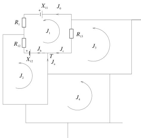
Figure 3. The planar network decomposed into simple loops with corresponding mesh fluxes. The details of the loop 1 are shown. The transition fluxes in outer branches are equal to the corresponding transition fluxes, *i.e.*  $J_0 = J_1$ . Transition fluxes in the branches common to the two simple loops is equal to the algebraic sum of the mesh fluxes of the corresponding simple loops, *e.g.*  $J_a = J_2 - J_3$ ,  $J_b = J_1 - J_2$ , and  $J_c = J_3 - J_1$ .
