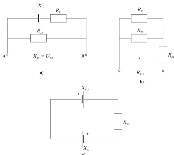
Figure 9. a) The part of the network which defines Thevenin's EMF,  $X_{T11}$ ; b) and resistance  $R_{T11}$ ; c) Replacement of the part of the network from the Figure 6 above the points A and B with Thevenin's source ( $X_{T11}$  and  $R_{T11}$ ).
