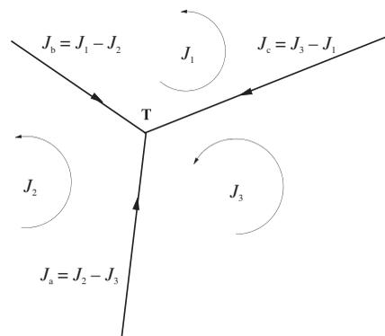
Figure 4. The blown up part of the network close to the point T from the Figure 3. Kirchhoff's law for fluxes is embedded into concept of mesh fluxes since  $J_a + J_b + J_c = 0$ .
