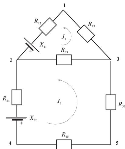
Figure 5. The electrical network equivalent to the chemical cycle kinetics of the enzyme-ligand complex close to the equilibrium constructed by means of Hill's diagram (see Figure 2). The values of the thermodynamic forces and resistances are given by expressions (5) and (22), respectively.
