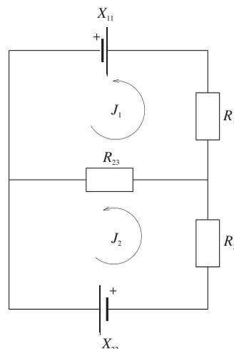
Figure 6. The electrical network from the Figure 5 after replacement of the resistance connected in the series with their equivalent resistances [see Eqs. (30) and (31)].
