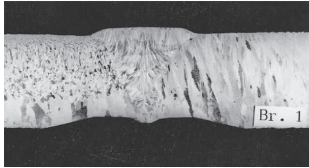
Figure 7 Macrostructure of repaired tube by welding
