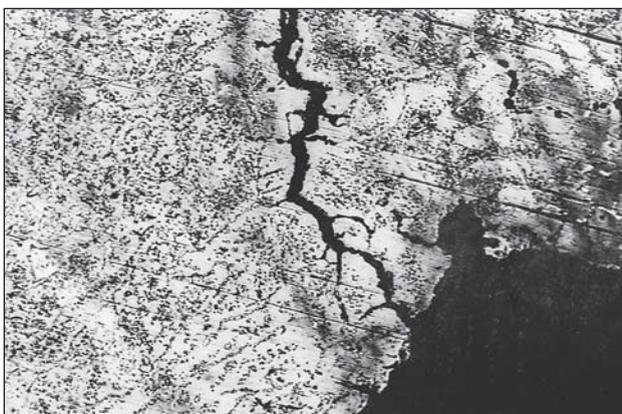
Figure 2 WHAZ cracks propagation (magnific. 10 x)
