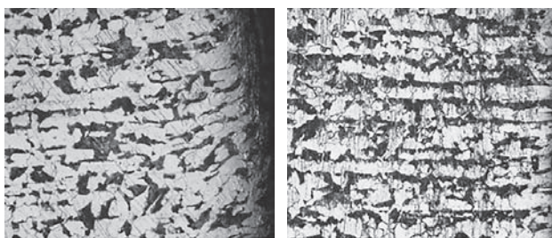
c) Wire Erosion cutting
