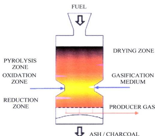
Figure 4b. Diagram of downdraft fixed bed gasifier
