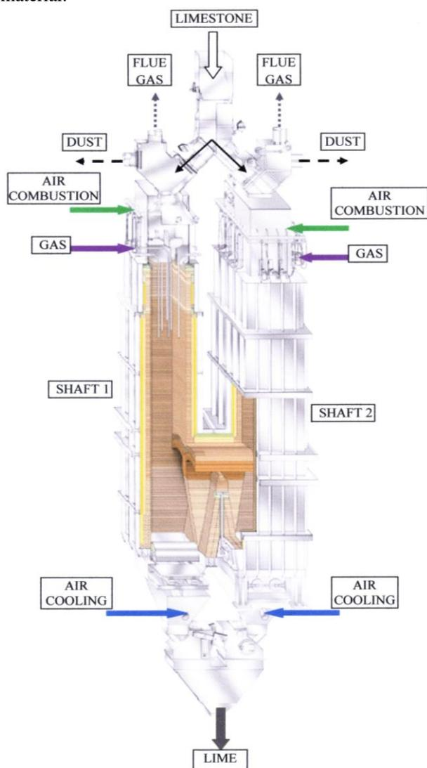
Figure 3. The scheme of Maerz furnace [1]
