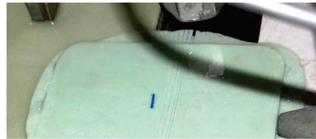
Figure 1 Cutting traces after disintegration of Palacos R+G® bone cement by continuous water jet with orifice diameter d = 0,1 mm
