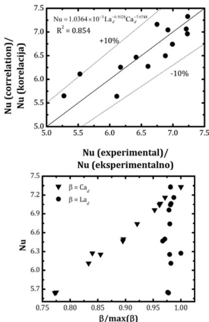
**Figure 9.** Comparison between  $Nu$  obtained experimentally and through an empirical correlation (top); and influence of dimensionless numbers  $Ca_d$  and  $La_d$  on the Nusselt number (bottom)
