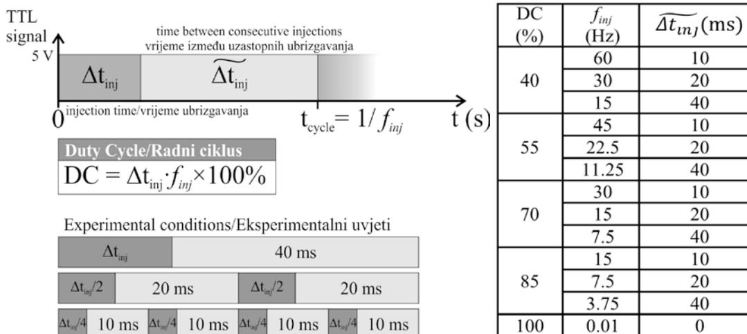
**Figure 1.** Illustration of the spray injection cycle and description of the experimental conditions considered for studying the effect of the spray intermittency on heat transfer.
