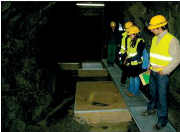
**Figure 6.** Niche with wells for the Mock-Up experiments.
