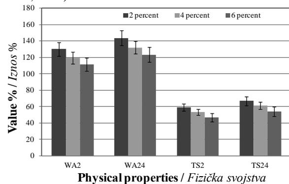
**Figure 3** The influence of oxidant percentage on water absorption and thickness swelling after 2 and 24-hour immersion
