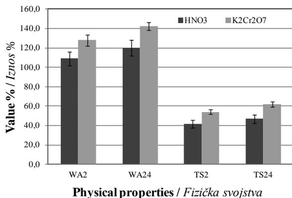
**Figure 2** Effect of oxidant type on water absorption and thickness swelling after 2 and 24-hour immersion in cold water
