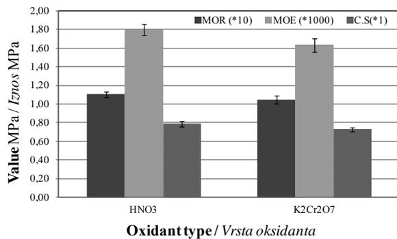
**Figure 1** Effect of oxidant type on modulus of rupture (*MOR*), modulus of elasticity (*MOE*) and *C.S* strength
