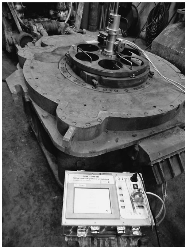
Figure 2 Measuring of crystallizer enclosure by MKL 100/420 system
