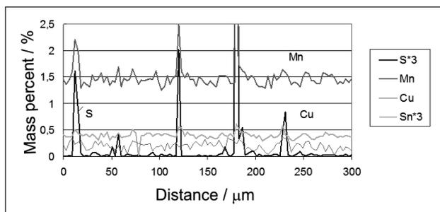
Figure 6 Example of concentration distribution for sulphur, manganese, copper and tin at the rapid cooled steel wrapper's surface obtained with microsonde
