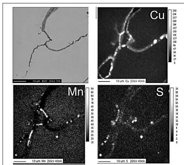
Figure 2 Reflection electron microscopy micrograph and mapping figures of a surface crack which occurred on a hot deformed steel block as well as enrichment with elements manganese, sulphur and copper [6]
