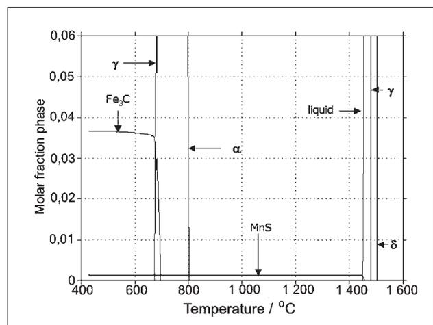
Figure 5 Thermocalc calculations of characteristic equilibrium phases for modified S355 steel depending on temperature
