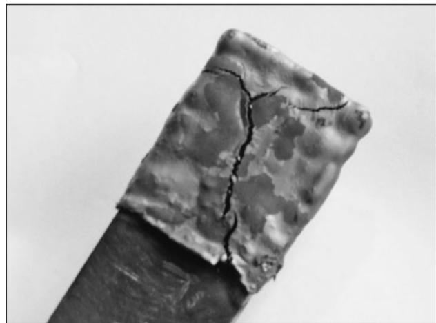
Figure 4 Appearance of rapid cooled steel wrapper on the copper plate after plunging
