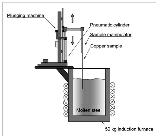
Figure 3 Schema of a half-automatic plunging machine for plunging of copper plate into molten steel
