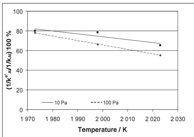
**Figure 3** Changes in the contribution of resistance related to evaporation to the overall process resistance depending on the pressure
