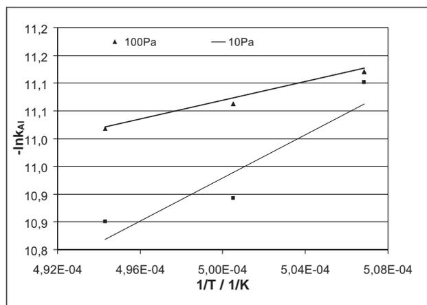
**Figure 4** The overall mass transport coefficient,  $k_{Al}$ , versus temperature
