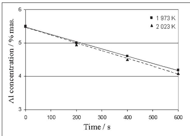
Figure 1 Changes in aluminium concentration during Ti-6Al-4V melting at 100 Pa, 1 973 K and 2 023 K
