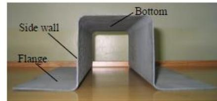
Figure 4. Ultra-high-strength boron steel stamping parts under high temperature.
