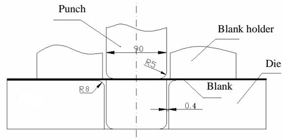
Figure 1. The sketch of the hot stamping bending dies.
