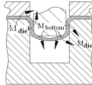
a) Springback caused by the forming force
