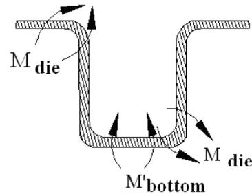
b) Springback caused by hot contact bending
