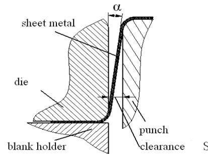
Figure 7. Diagram of the wedge angle  $\alpha$ .
