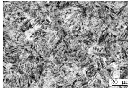
Figure 5. Microstructure of ultra-high-strength boron steel stamping parts.
