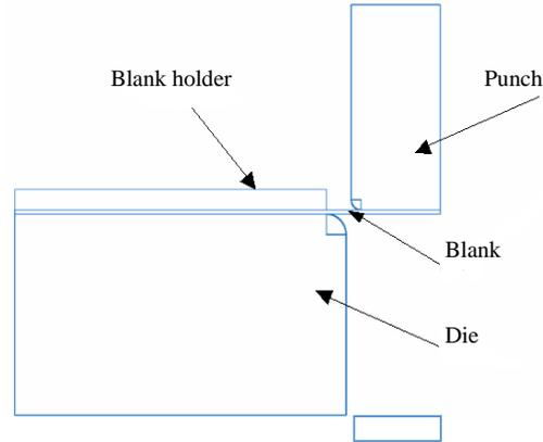
Figure 3. The geometric model of the U-shaped parts achieved by hot contact bending.
