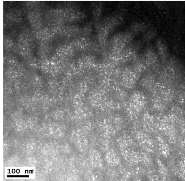
Figure 4. Dark-field electron microstructures for (111) superlattice spots of DO3-Fe<sub>3</sub>Al phase aged at 565°C for 60min
