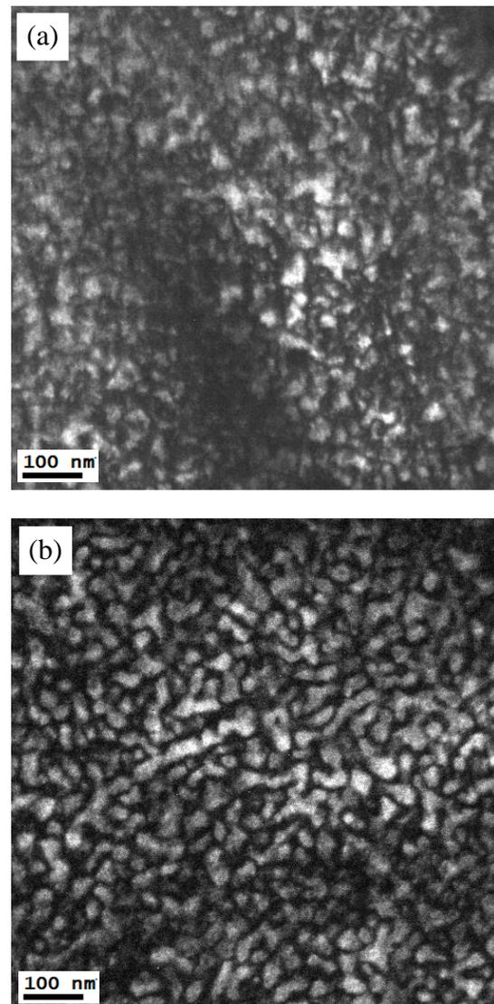
Figure 3. Dark-field electron microstructures for  $(100)$  superlattice spots of B2-FeAl phase aged at  $565^\circ\text{C}$  for variation/varying time (a) 1min; (b) 3min.
