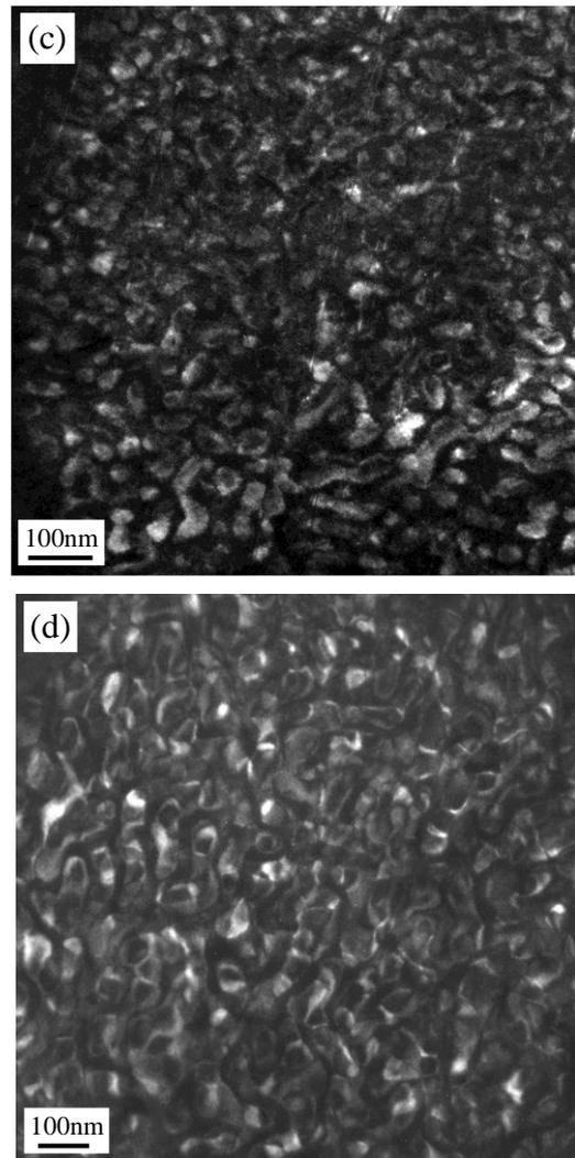
Figure 5. Dark-field electron microstructures for (111) superlattice spots of DO3-Fe<sub>3</sub>Al phase aged at 520°C for variation time (a) 5min, (b) 10min, (c) 60min, (d) 120min.
