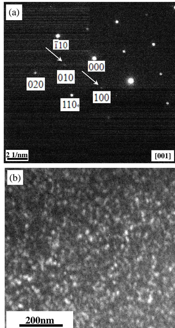
Figure 2. The microstructure of the Fe-23Al alloy solution-treated at 800°C for 0.5h by TEM (a) diffraction pattern for [001] zone axis of  $\alpha$ -Fe, (b) dark image of B2-FeAl phase for (100) superlattice spots (equivalently, (200) for DO3-Fe<sub>3</sub>Al phase).
