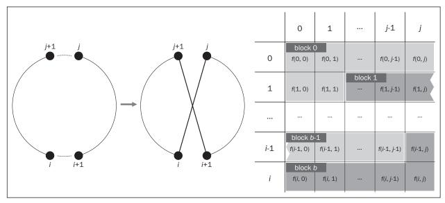
Figure 3 - Left: 2-opt, Right: implementation on CUDA architecture
