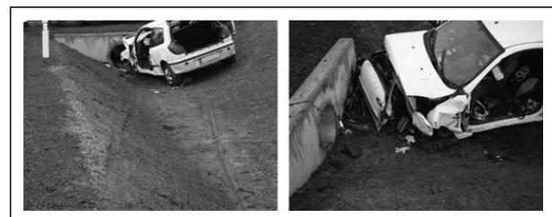
Figure 4 - Collision of an automobile with an access bridge – car body deformation
