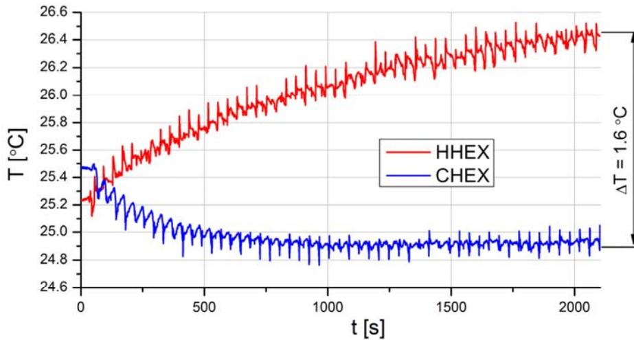
Fig. 3 Temperature difference between the hot and the cold heat exchanger [16]
