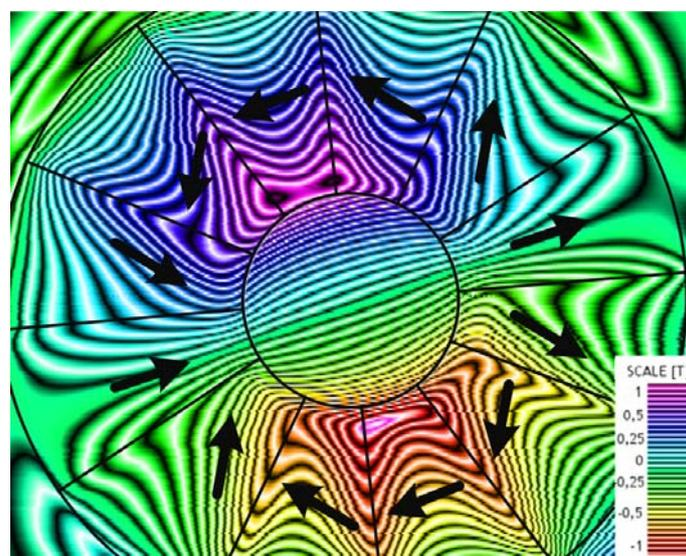
Fig. 7 Magnetic field distribution on the surface of the Halbach array - value of the Z component of the magnetic field vector, perpendicular to the surface. Contours of the magnets are also marked
