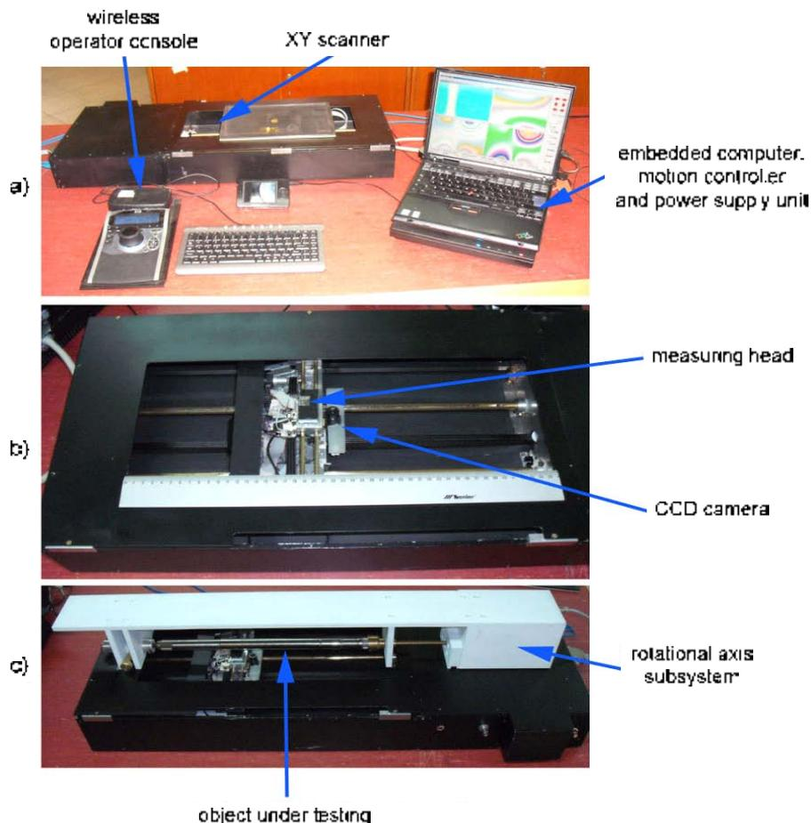
**Fig. 5** General view of the Magscanner-Maglab System: scanner setup (a), measuring area (b), subsystem for axisymmetric measurements (c) [17]
