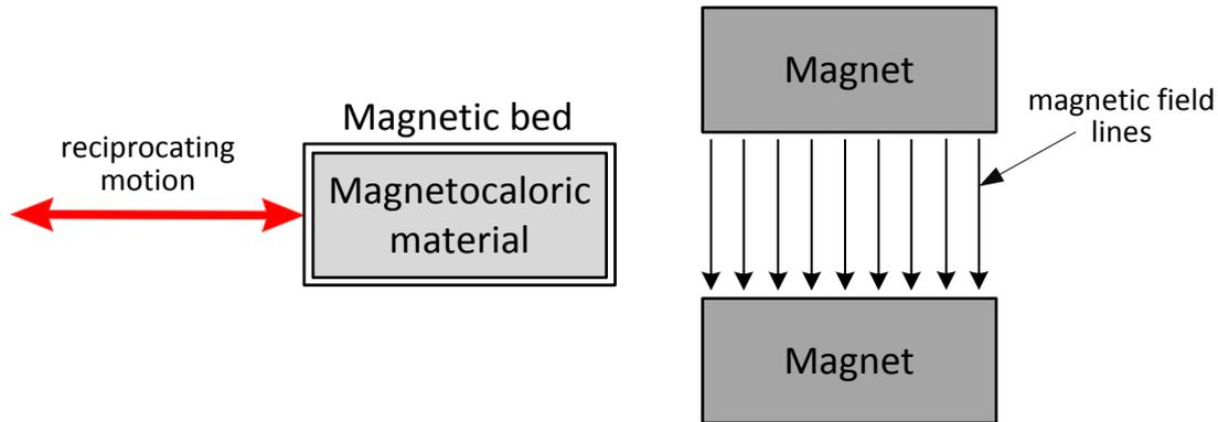
**Fig. 1** Cyclical magnetisation and demagnetisation of a magnetocaloric material, caused by the reciprocating motion of a magnetic bed
