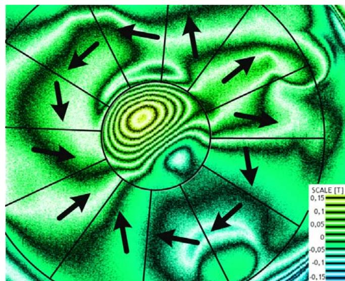
**Fig. 11** Magnetic field distribution on the surface of the magnetic screen when the Halbach array is placed under the screen - value of the Z component of the magnetic field vector, perpendicular to the surface. Contours of magnets are also marked
