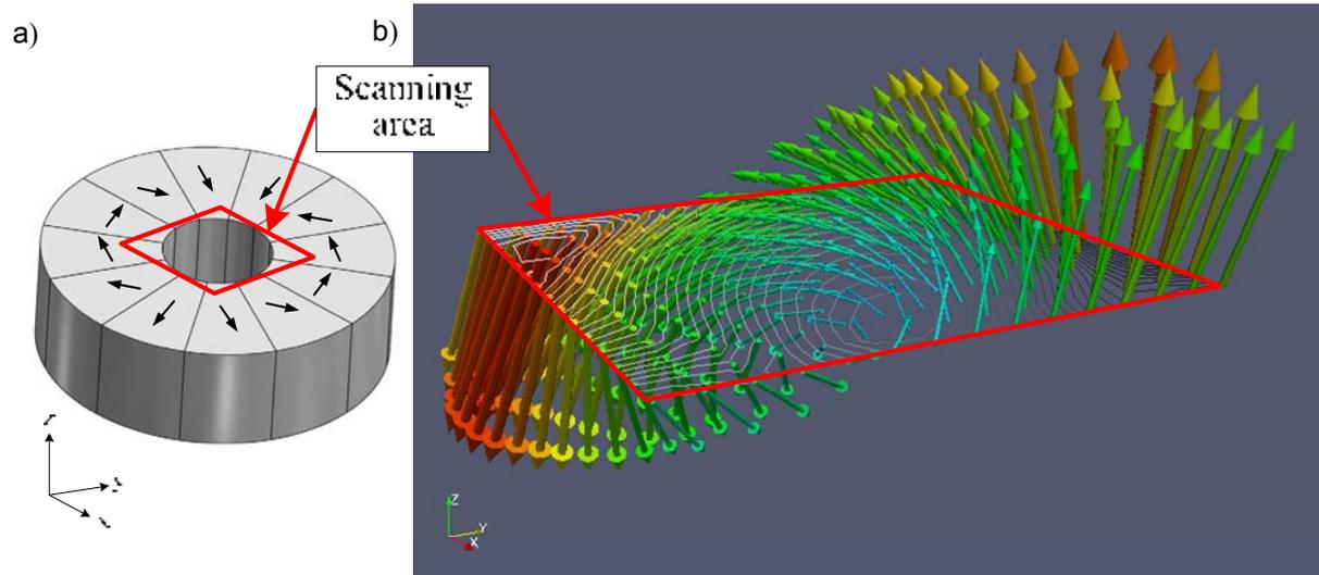
**Fig. 8** Model of the Halbach array with a marked scanning area (a) and magnetic field vector distribution on the surface of the Halbach array in the scanning area (b)
