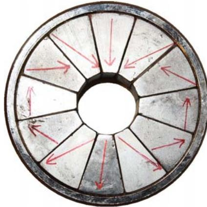
Fig. 6 Photograph of the used Halbach array [16]
