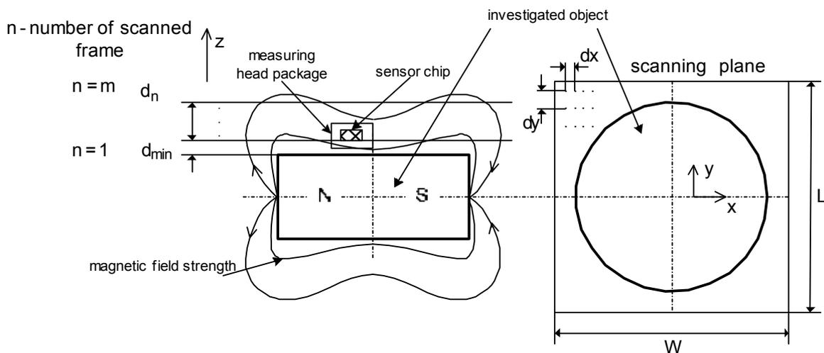
Fig. 4 Idea of the magnetic field scanning [17]
