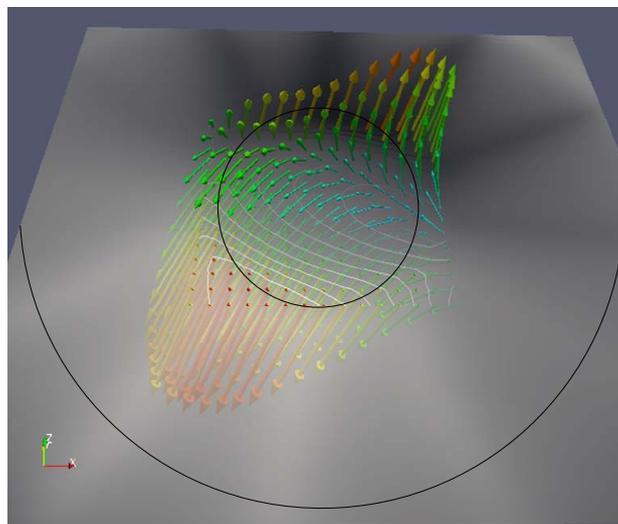
**Fig. 9** Magnetic field distribution with a marked contour of the Halbach array
