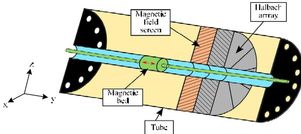
**Fig. 10** Cross-sectional view of the tube
