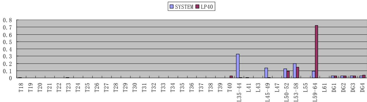
Figure 7. Components failure probabilities on the condition of system or load point 40.
