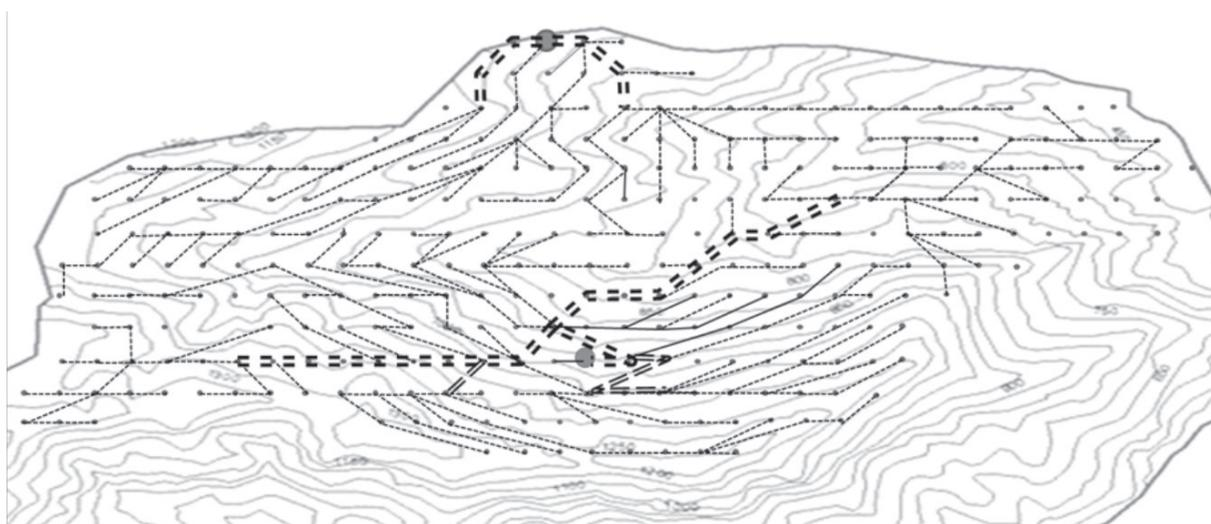
**Fig. 10** Solution showing the road and related access spurs (*Rfact* = 0.40, 2 Exit Points)
