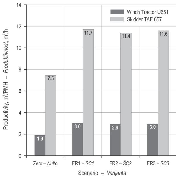
**Fig. 5** Timber extraction productivity, by infrastructure scenario
