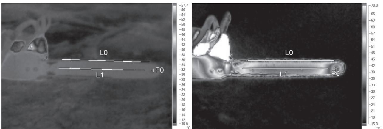
**Fig. 3** Infrared snapshots of the STIHL cutting system, left – 1<sup>st</sup> interval, right – 4<sup>th</sup> interval
