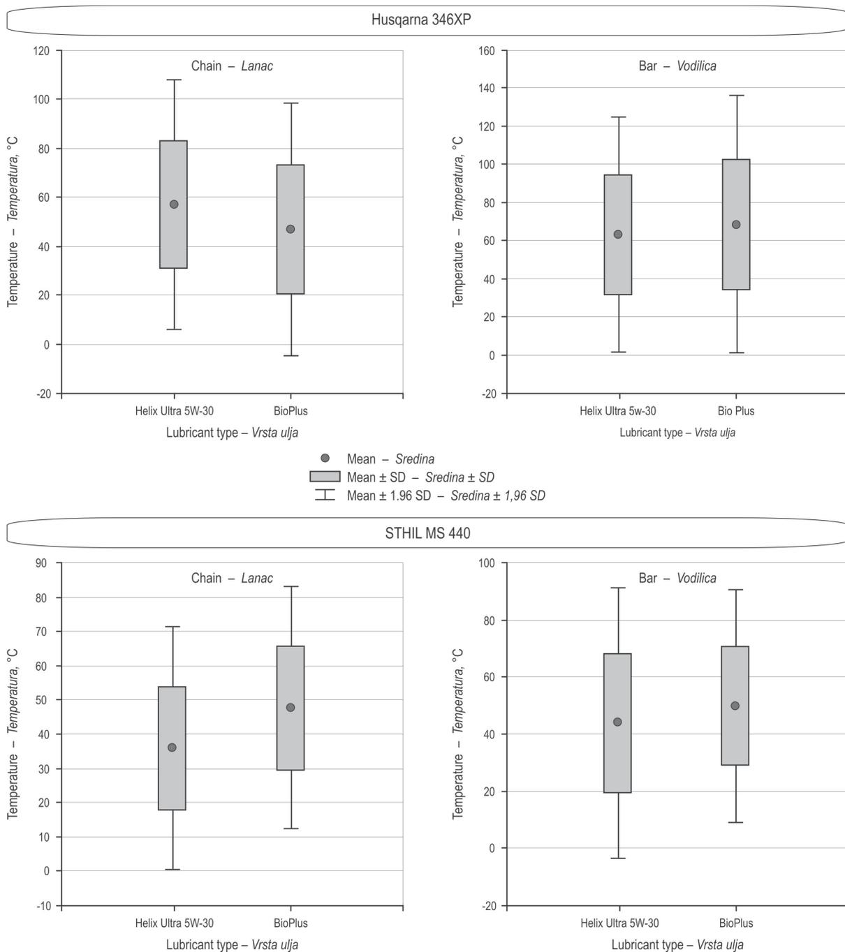
Fig. 4 Box charts showing temperature variability of cutting systems with both chainsaws and lubricant types
