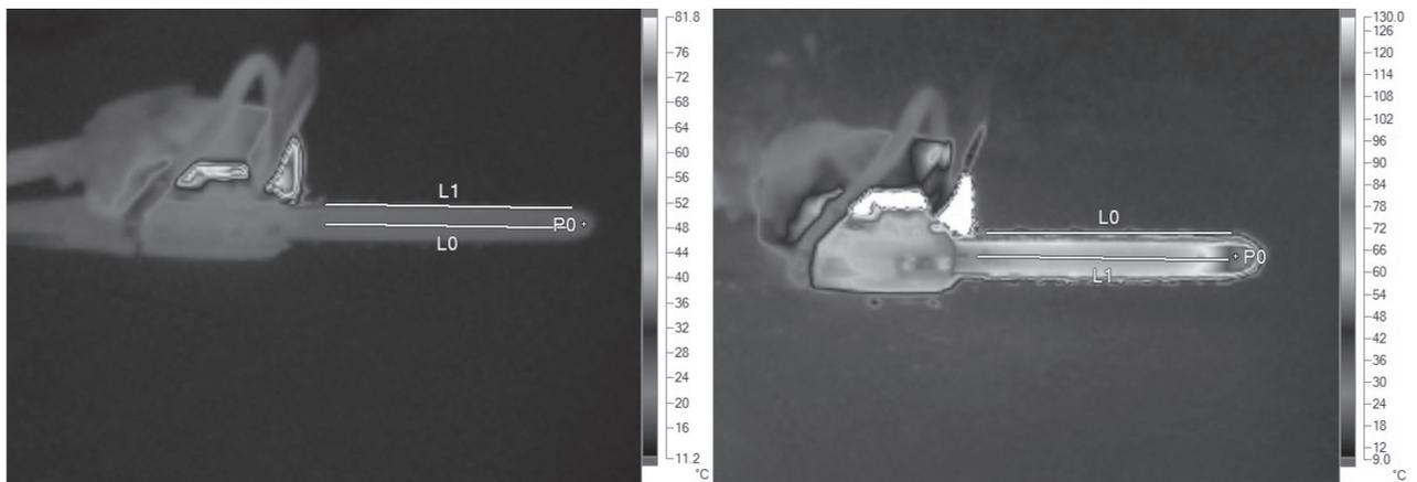
**Fig. 2** Infrared snapshots of the Husqvarna cutting system, left – 1<sup>st</sup> interval, right – 4<sup>th</sup> interval
