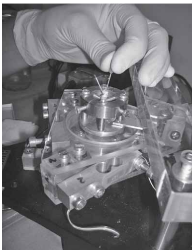
Fig. 2. Lateral condensation of gutta-percha cones in the tooth attached to the measurement device
