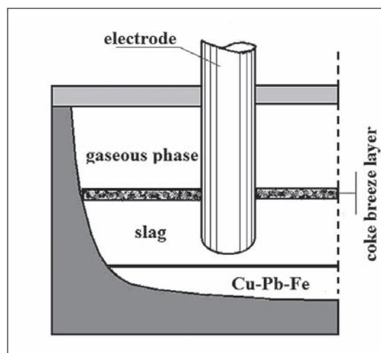
**Figure 1** A demonstrative schematic diagram of phases in the electric furnace during a process of flash slag melting
