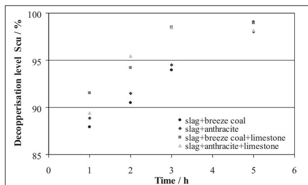
Figure 4 Slag decopperisation level change versus reduction time
