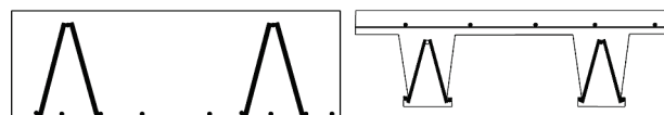
Figure 12 Cross-section of the reinforced slab made with SSLC (left) and ordinary semi-precast FERT floor slab (right)
