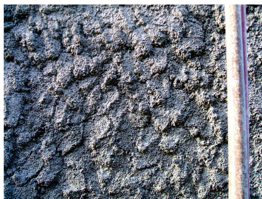
Figure 4 Fresh lightweight mortar made with ground recycled EPS aggregate during its application
