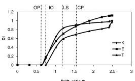
Drift ratio % Figure 5 Variations of structural damage indexes at different performance levels of the six-story frame
