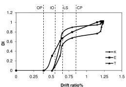
Figure 6 Variations of structural damage indexes at different performance levels of the twelve-story frame
