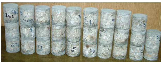
Figure 8 View of a part of cores, prepared for testing
