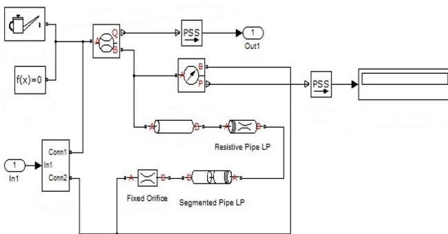
Figure 4. Diagram of fuel lines and fuel pump
