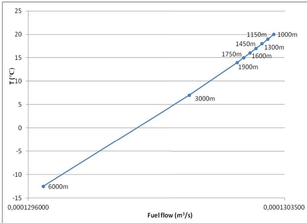
Figure 6. The graph of changes depending on the temperature of the fuel flow and the height of flight
