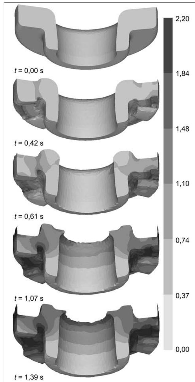
**Figure 3** Workpiece shape changes and effective strain distribution when  $v = 15$  mm/s and  $F = 4$  000 kN
