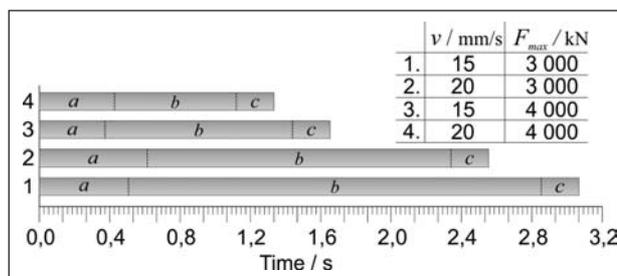
**Figure 6** Duration of the orbital forging stages, depending on the velocity  $v$  and upper limit of the forming force  $F_{max}$ ; description in the text
