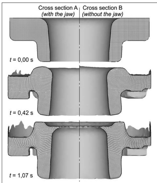
**Figure 4** Flow net deformation in cross section of the workpiece, the same case as in Figure 3
