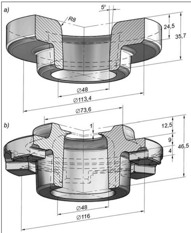
**Figure 1** Shape of the investigated part: a) preform, b) hollow forging of a jaw coupling sleeve-disk
