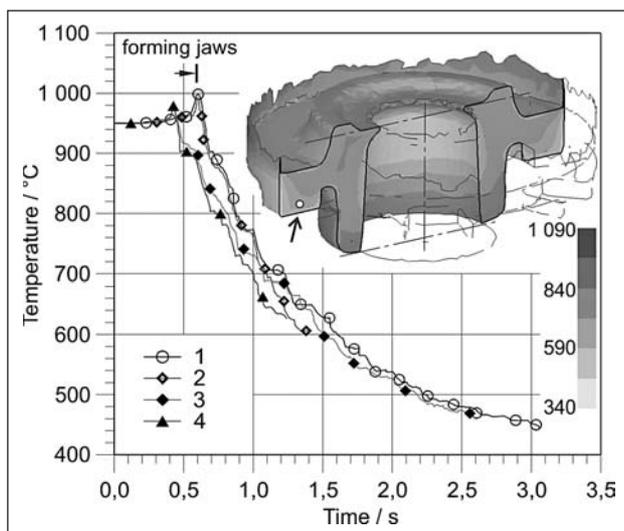
**Figure 7** Temperature change versus time at a selected point in the workpiece; the meaning of the curves is given in Figure 6
