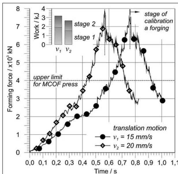
**Figure 5** Forming force  $F$  versus time of the process and calculated work performed by the dies
