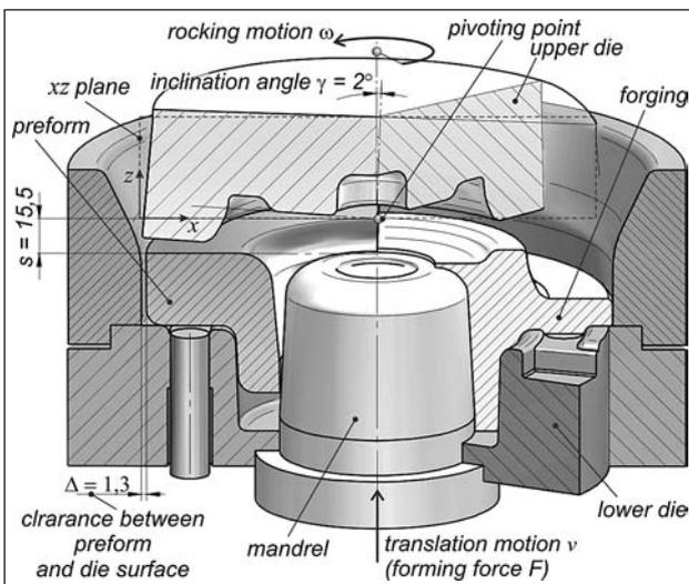
**Figure 2** Design of the orbital forging process for producing a jaw coupling sleeve-disk
