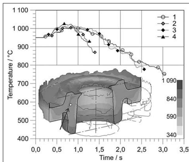
**Figure 8** Temperature change versus time at a selected point in the workpiece; the meaning of the curves is given in Figure 6
