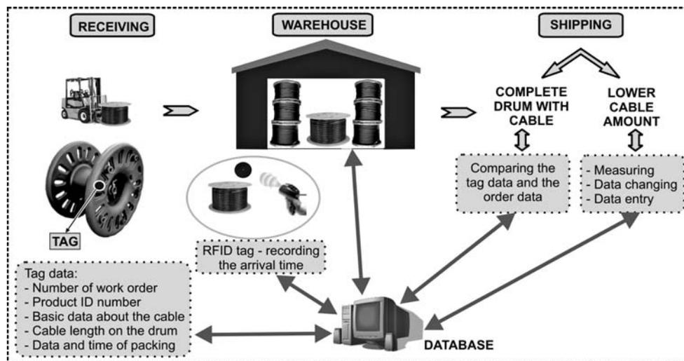
Figure 4 The application of RFID technology in cable storage
