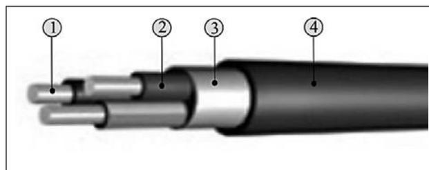
**Figure 1** Product composition: 1 – Cu conductor, 2 – PVC insulation, 3 – unvulcanized tire filling and 4 – PVC sheath
