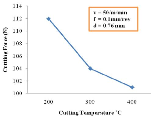
Figure 3. The effect of cutting temperature on the cutting force.
