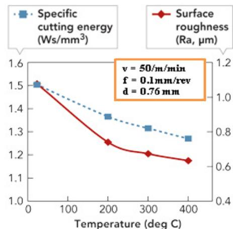
Figure 5. The Effect of temperature exerted on Specific cutting energy and surface roughness [58].
