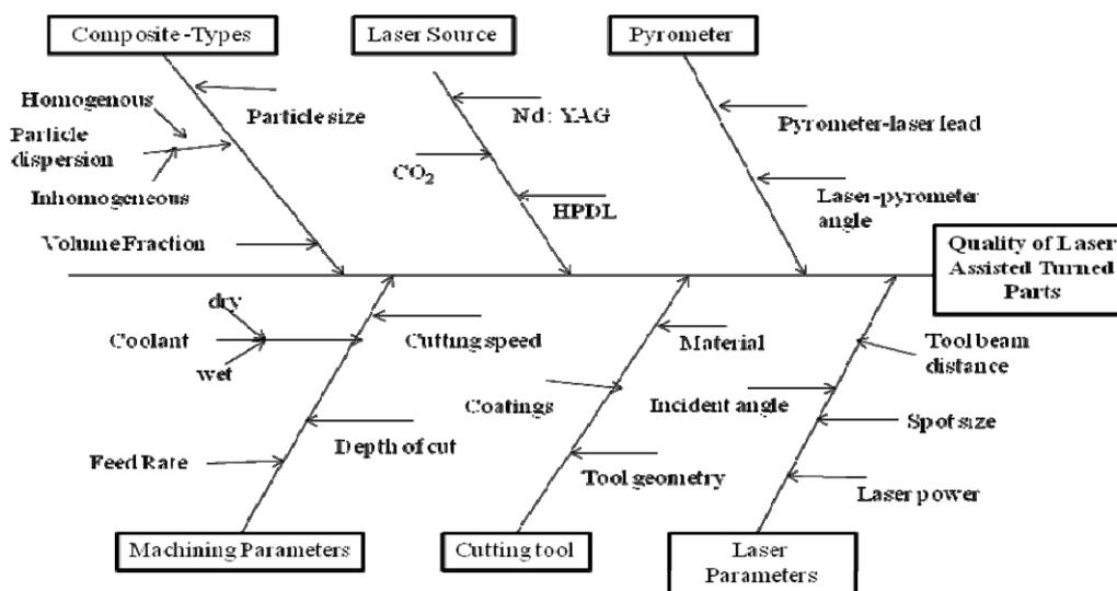
Figure 6. Ishikawa cause-effect diagram of a laser assisted turning process.
