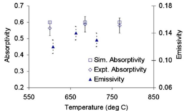
Figure 2. The effect of temperature on absorptivity and emissivity [58].
