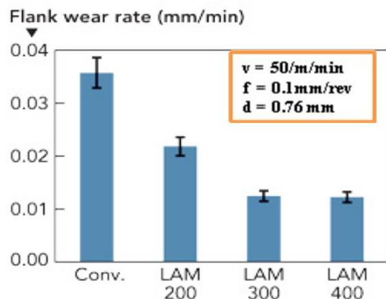
Figure 4. Tool wear vs. temperature [58].
