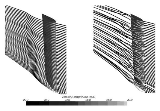
Figure 6. The flow around the blades at an AoA of  $25^{\circ}$ , shaded by velocity magnitude (ms<sup>-1</sup>).
