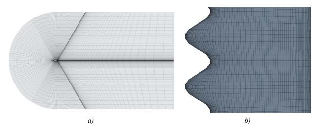
Figure 3. Numerical mesh displayed on; a) the upper wall, b) the blade surface.
