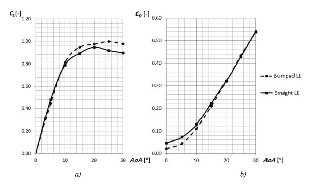
*Figure 5. Coefficients a) lift*  $C_L$  *and b) drag*  $C_D$  *as curves for both blade LE types over the AoA range.*
