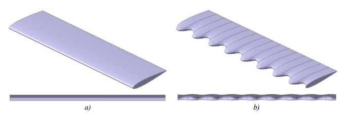
Figure 2. Leading edge of the two blade models: a) straight LE, b) bumped LE and surface.
