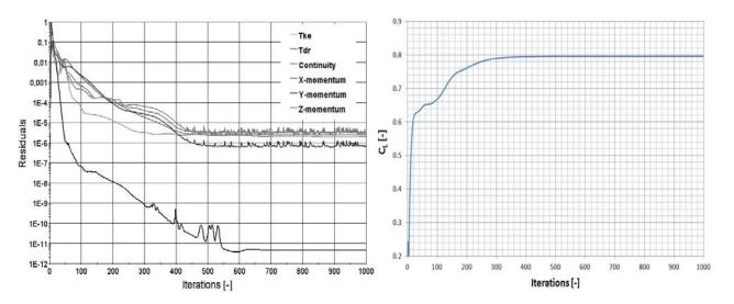
Figure 4. Convergence of residuals(left) and monitored values of lift coefficient (right) during iteration.
