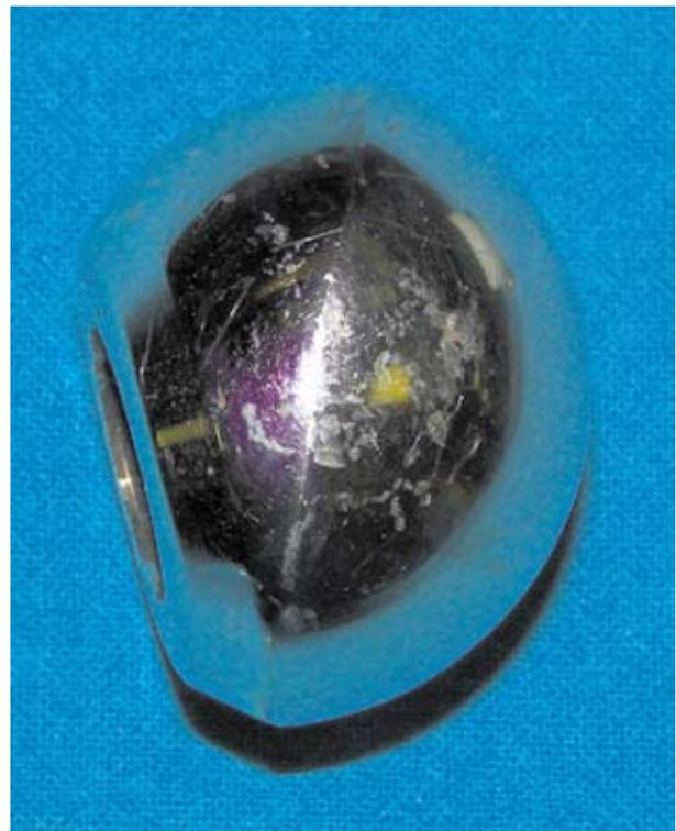
*Fig. 4. Elliptic head as a result of wear.*
