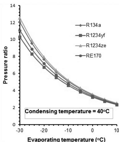
Figure 7. Effect of the evaporating temperature on the pressure ratio
