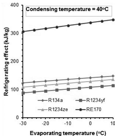
Figure 3. Influence of the evaporating temperature on the refrigerating effect
