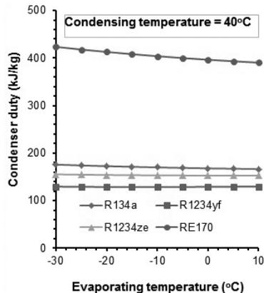
Figure 4. Variation of the condenser duty with evaporating temperature
