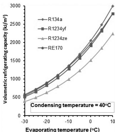
Figure 8. Effect of the evaporating temperature on the volumetric refrigerating capacity
