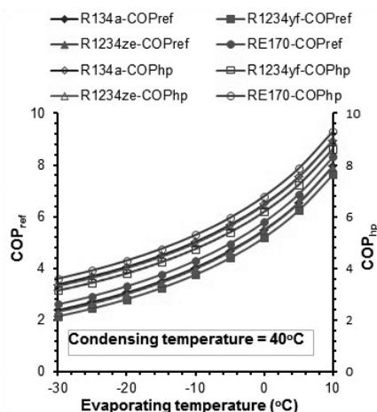
Figure 6. Variation of the coefficient of performance of refrigeration ( $COP_{ref}$ ) and heat pump ( $COP_{hp}$ ) with evaporating temperature
