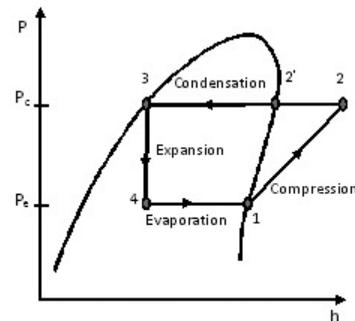
Figure 1. Conventional refrigeration cycle on p-h diagram
