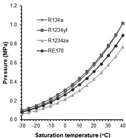
Figure 2. Variation of pressure with saturated liquid temperature
