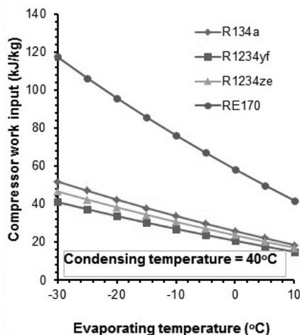
Figure 5. Compressor work input versus evaporating temperature
