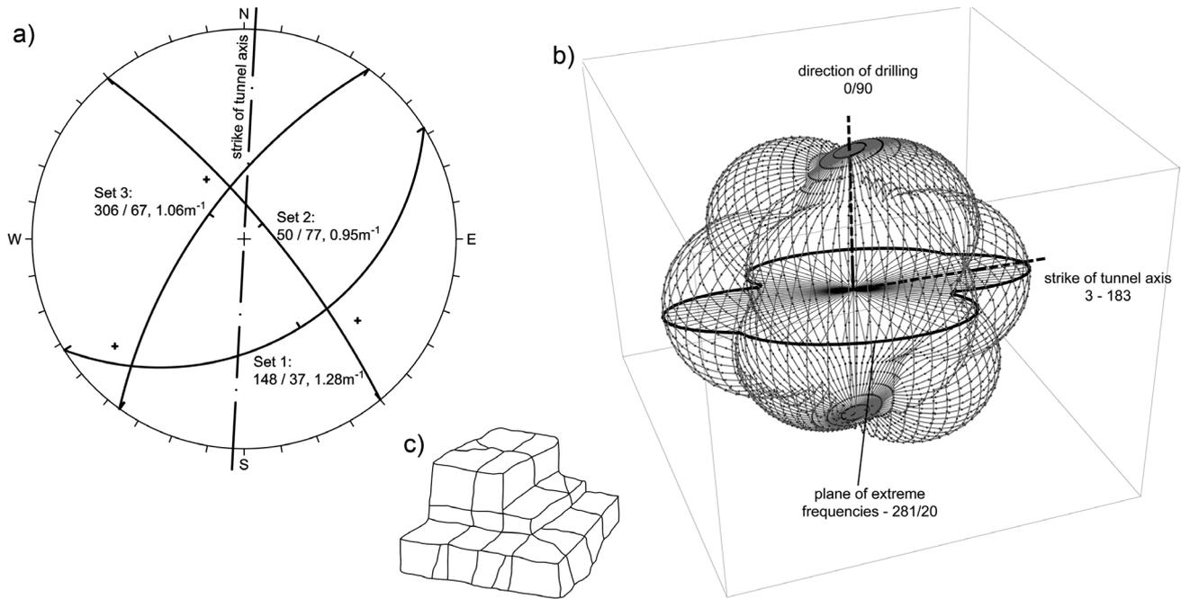
**Figure 6:** The "Mala Kapela" Tunnel – structural unit A (3 sets): a) Equal angle lower hemispherical projection of example data, b) three-dimensional locus of discontinuity frequency with plane of extreme (range) frequencies, c) euidimensional blocks.
