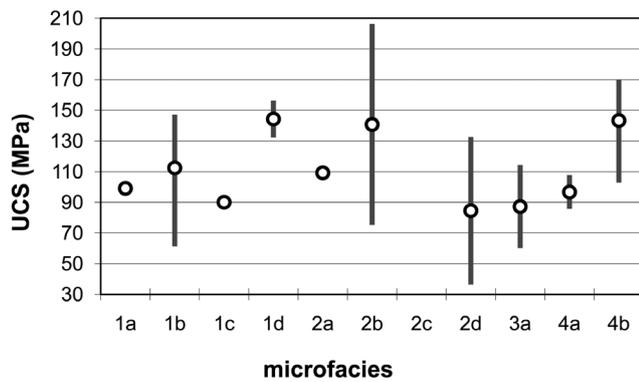
**Figure 4:** The ranges and averages of uniaxial compressive strength (UCS) for particular microfacies (19 samples in total). Zagreb-Split motorway, section Tunnel Sveti rok-Maslenica.
