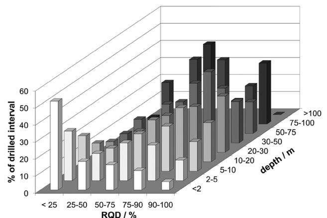
Figure 12: The histogram of RQD index values in relation to the depth of the drilled interval from boreholes across AdCP.
