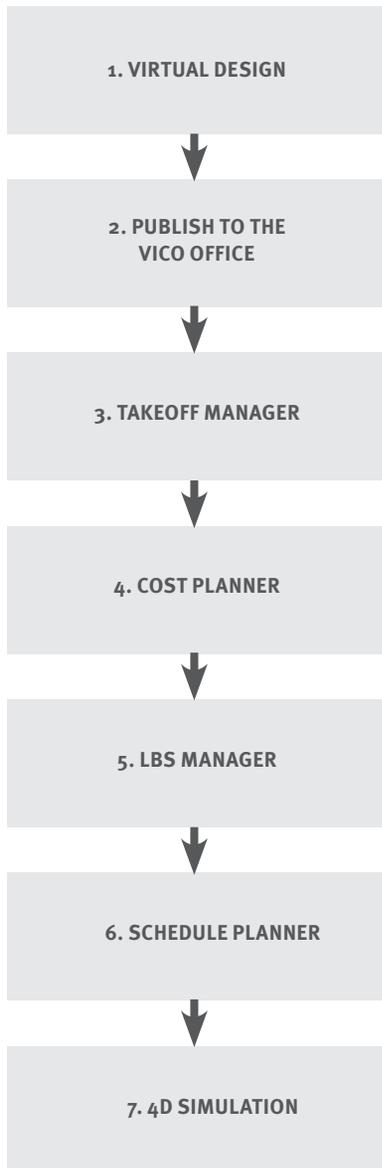
**Figure 2. Flowchart of work steps for BIM based time and cost planning of construction project**
