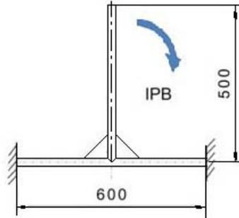
Fig. 3 “T” connection dimensions and load type
