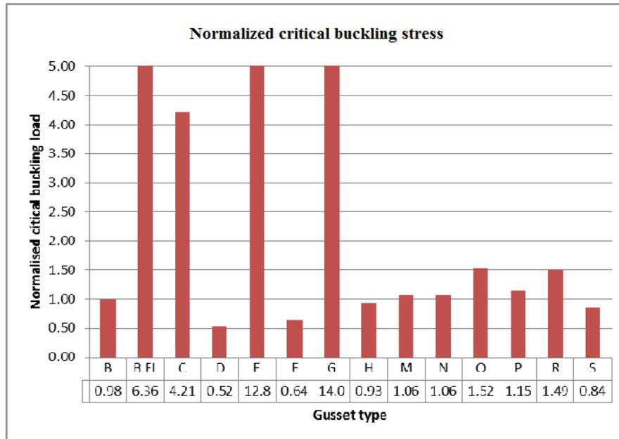
Fig. 7 Normalised critical buckling load for studied gussets
