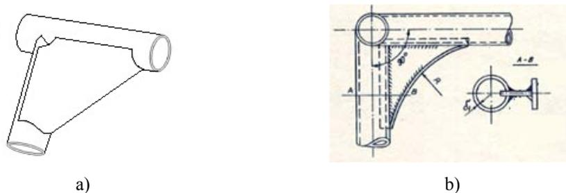
**Fig. 2** a) Closed gusset (“U” shaped section) [19]; b) Welded flange gusset [8]
