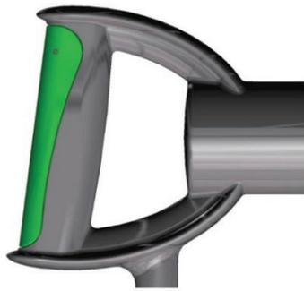
Figure 12 Virtual model of redesigned handle
