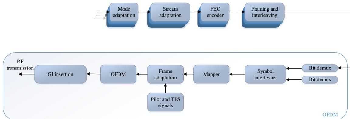
Fig. 1. DVB-SH-A transmission block diagram [1].
