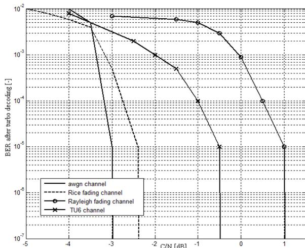
Fig. 7. Bit Error Rate for communication over the different channel models with system parameters: QPSK1/5, 2K OFDM, GI = 1/16 and for TU6  $v = 50$  km/h.
