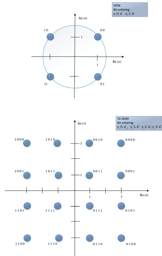
Fig. 3. QPSK and 16-QAM mapping [1].
