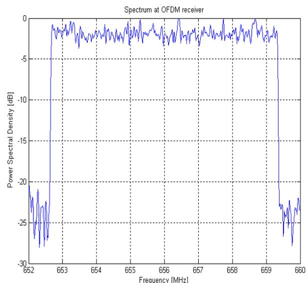
Fig. 4. Spectrum of OFDM signal (gained with simulation model).
