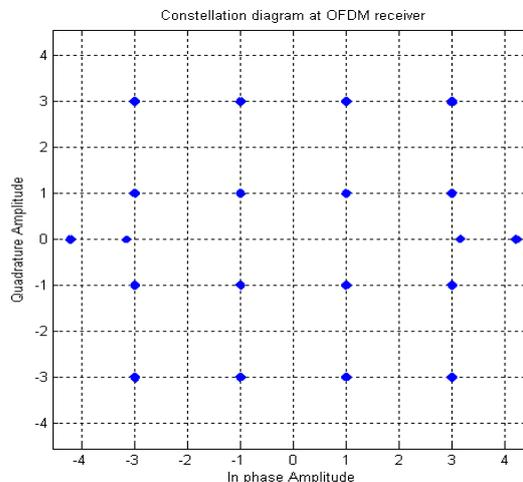
Fig. 5. Constellation diagram for the 16-QAM at  $C/N=20$  dB.
