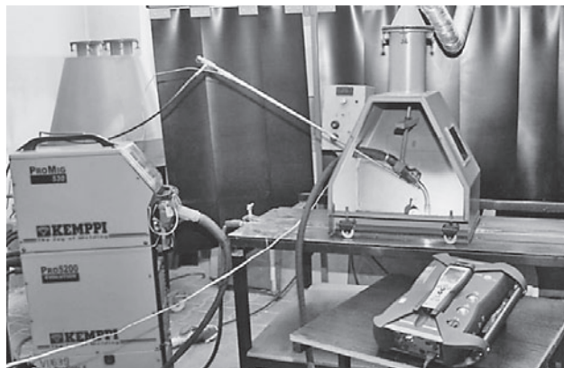
Figure 1 Research station for testing fume and gas emission while MIG/MAG arc weld brazing
