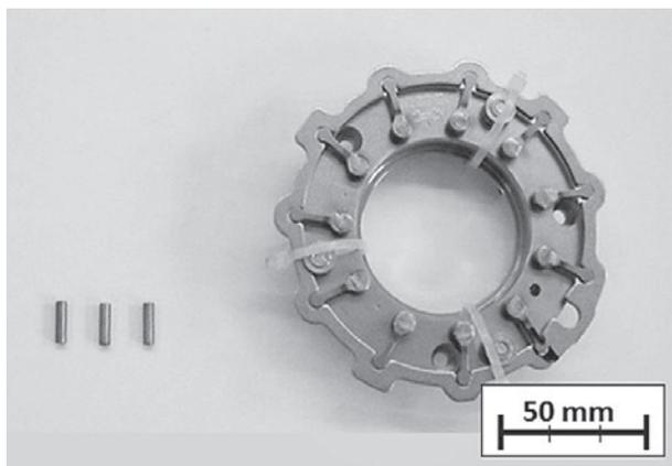
**Figure 4** The axles of the pressure control regulator rollers before the test
