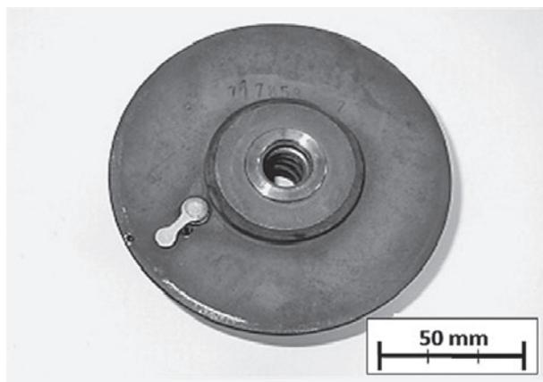
**Figure 3** Turbine lid. The arrow indicates the sealing made of the alloy based on FeAl intermetallic phase matrix.
