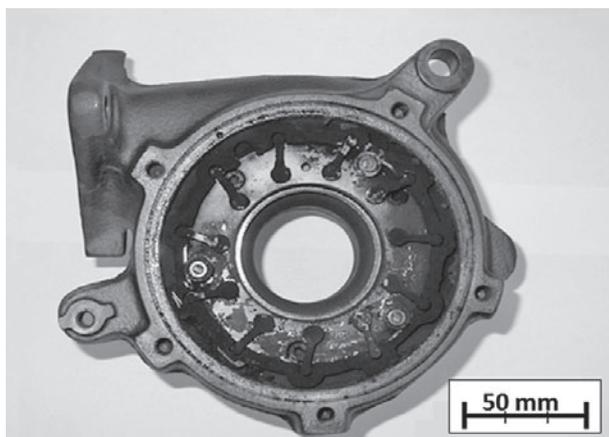
**Figure 5** The turbine after 20 000 km
