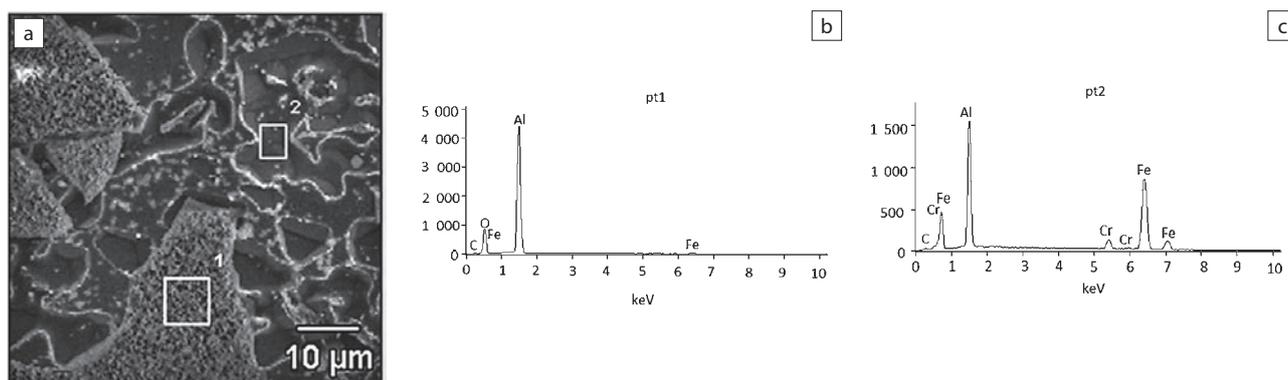
**Figure 2** X-ray energy spectra (EDS): a - state surface, b - analysis in point 1, c - analysis in point 2
