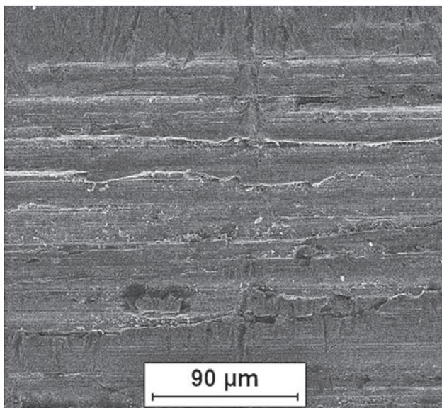
**Figure 6** Surface of the roller axle of the control unit made of FeAl alloy. SEM
