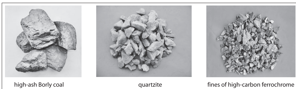
Figure 1 Charge components of aluminum silicon-chrome (FASCh) process
