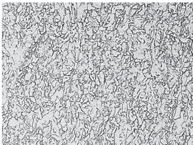
Figure 3 Microstructure of the steel no. 350 – the end of rolling at temperature 780 °C, cooling rate is 30 °C/s; mag. x1000
