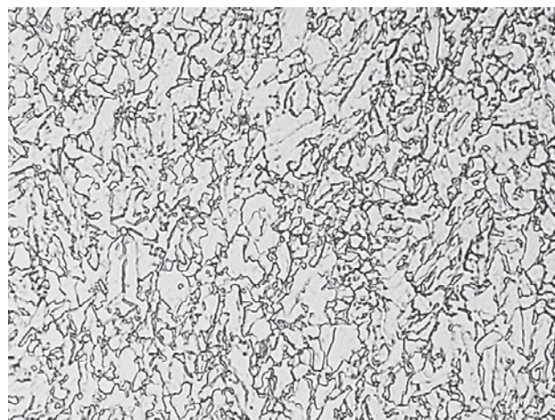
Figure 5 Microstructure of 355 steel cooled to temperature 300 °C with cooling rate 10 °C/s, mag. x1000
